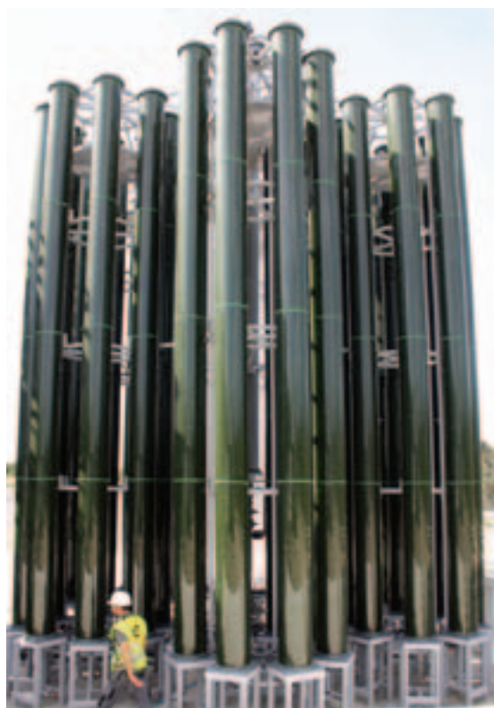
Photo 9.2 Near Alicante, Spain, tubes filled with microscopic algae turn CO 2 and sunlight into synthetic oil
