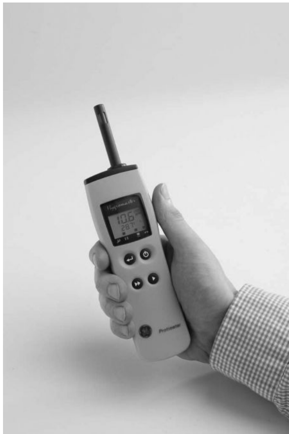
Figure 2.5 'Protimeter Hygromaster' hygrometer (courtesy GE Sensing Infrastructure, Inc)
