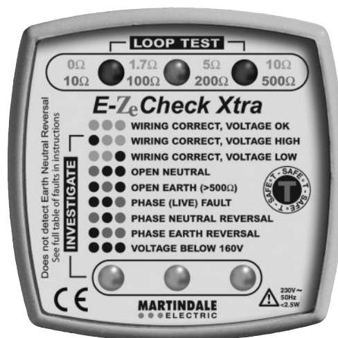
Figure 2.8 Earth loop impedance socket tester (courtesy of Martindale-Electric)
