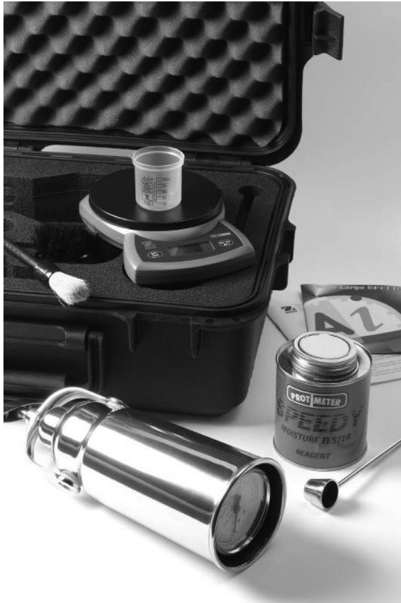
Figure 2.7 'Protimeter Speedy Moisture Tester' carbide meter (courtesy GE Sensing Infrastructure, Inc)
