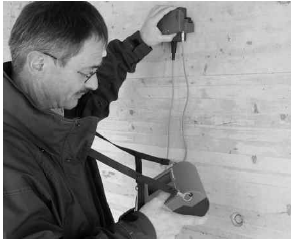
Figure 2.6 Reinforcement detector and analysis and cover meter (courtesy of Proceq)
