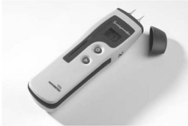
Figure 2.3 ‘Protimeter Surveymaster SM’ moisture-reading meter (courtesy GE Sensing Infrastructure, Inc)
