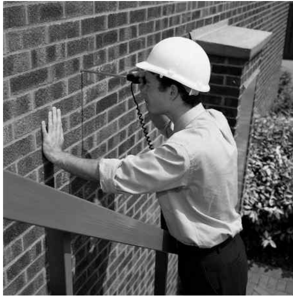
Figure 2.4 Surveyor using a borescope (courtesy of Olympus Industrial)
