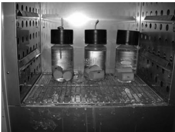
Figure 3.18 Water absorption test.
