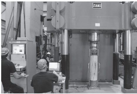
(a) MTS test frame with data-acquisition system
