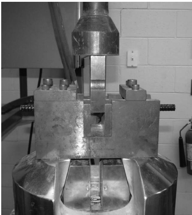
Figure 3.5 Typical transverse shear test setup.
