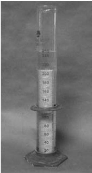
Figure 3.1 Measurement of the cross-sectional area of an FRP bar by the Archimedes principle.
