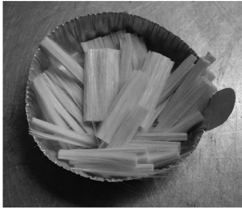
Figure 3.15 Typical GFRP bar sample at the end of the ignition loss test.
