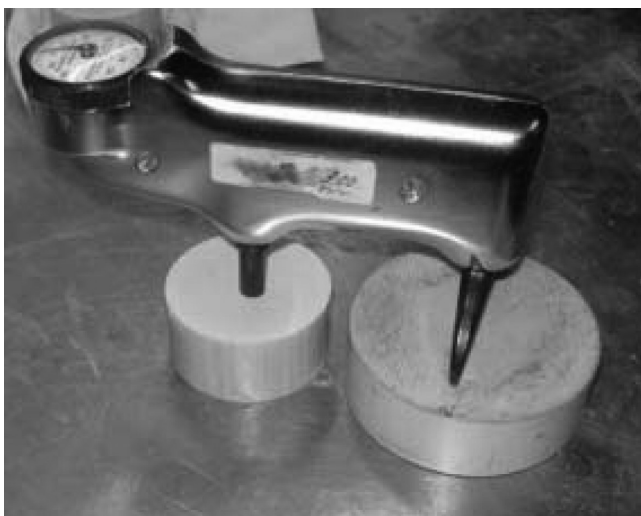
Figure 3.17 Barcol hardness test setup and apparatus.
