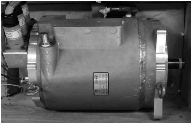
Figure 7.18: 100kW fuel cell EV motor (Hyundai Motor Company).
