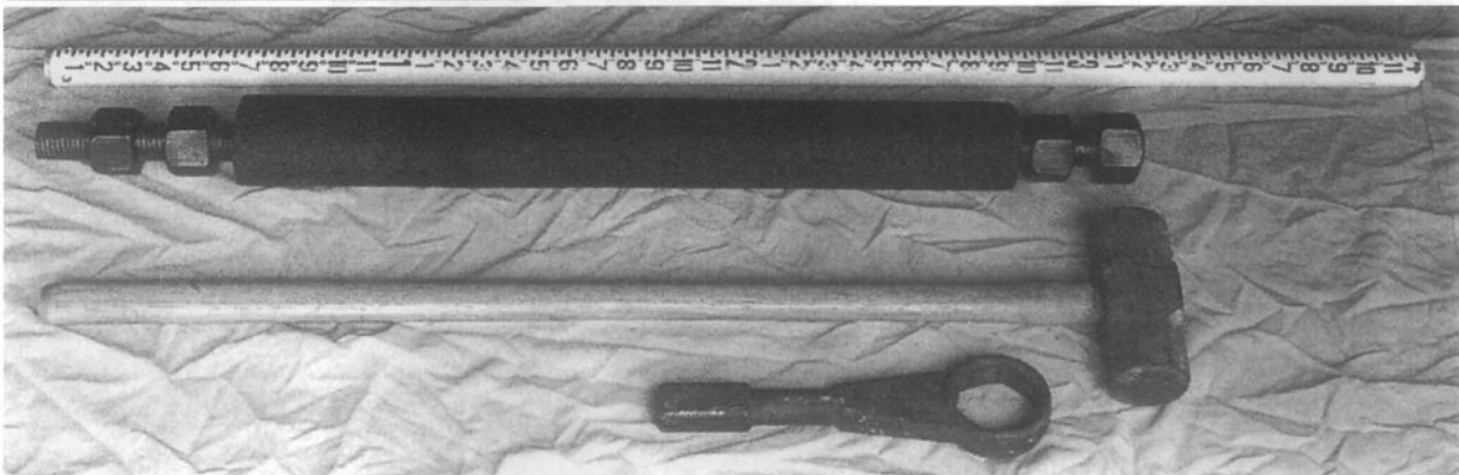
Figure 25-11 The 1 1/2" Ø bolt in an epifoam insulation sleeve is shown here with a 10 Lb. hammer and hit wrench. The surveyor's rod is used for reference.
