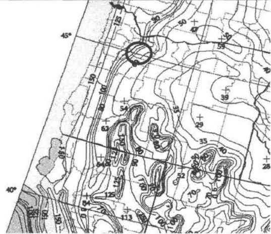
Figure 39-2 This is the map for the 0.2 second spectral response acceleration.
