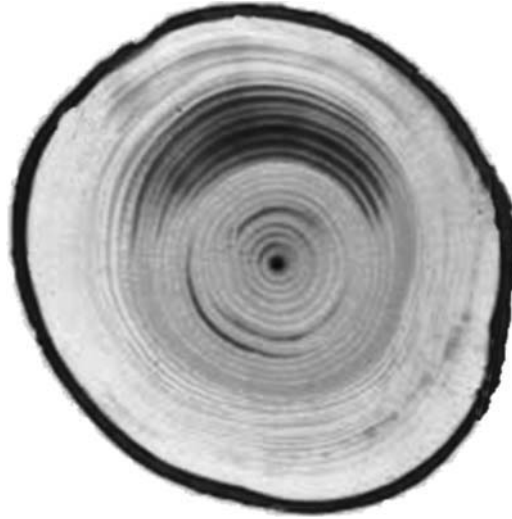
Fig. 1.2. Compression wood (dark patch).
