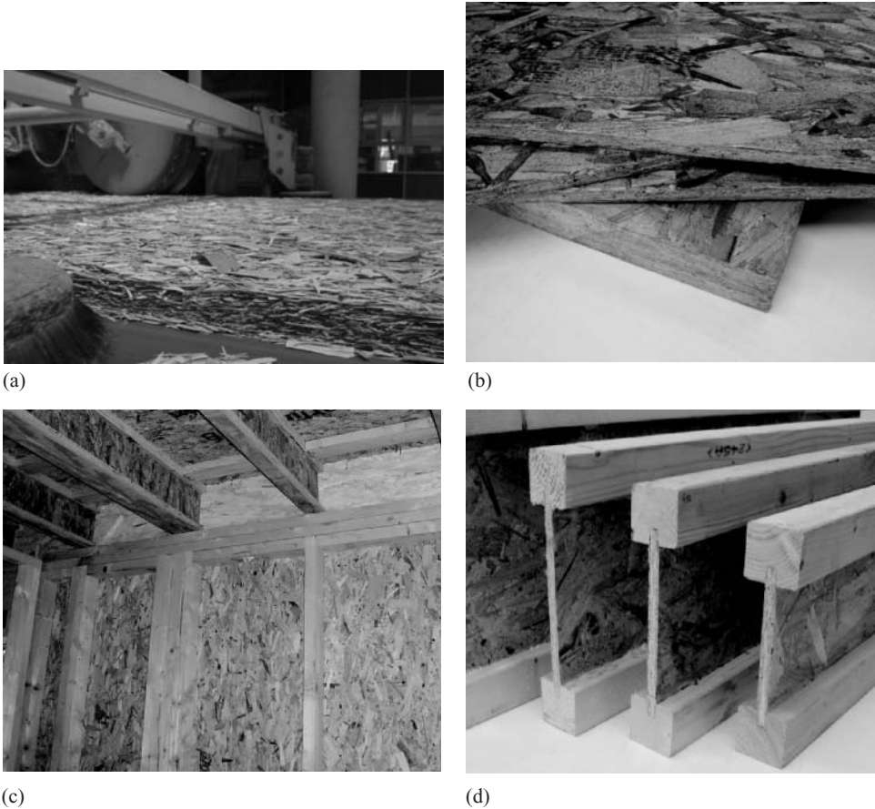
Fig. 1.14. OSB: (a) production before the press (photo courtesy of Wikipedia Foundation); (b) and (c) OSB boards and wall panels; (d) OSB webs in I-joists.
