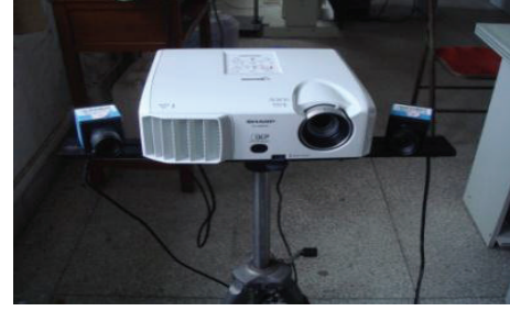
FIGURE 4: Picture of the 3D surface profile measurement system.
