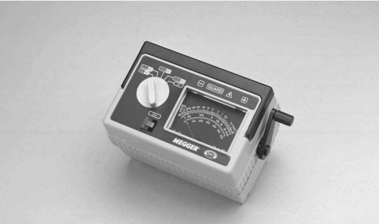
Figure 25-4 Hand-crank megger. (Courtesy of Biddle Instruments)
