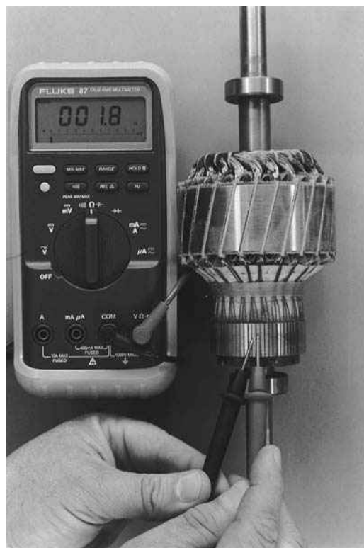
Figure 1-13 Digital ohmmeter being used to measure resistance.
