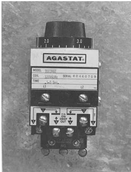
Pneumatic off-delay timer. A microswitch has been added to the bottom to supply instantaneous contacts for the timer.
