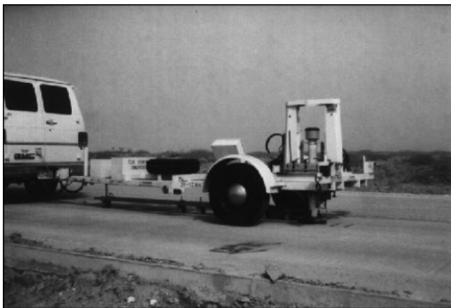
Figure 20.2 Falling weight deflectometer. (Photo by the author.)
