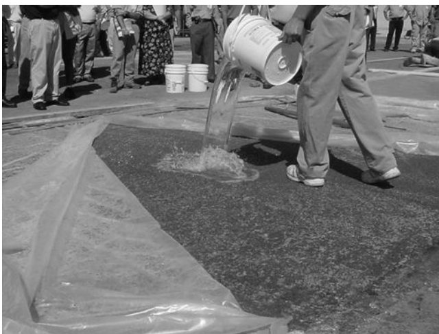
Figure 2.11 Permeability of a pervious pavement demonstration project—Cleveland, Ohio. (Photo by author.)
