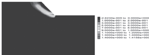
(b) with FLAC 3D (plastic shear strain)
