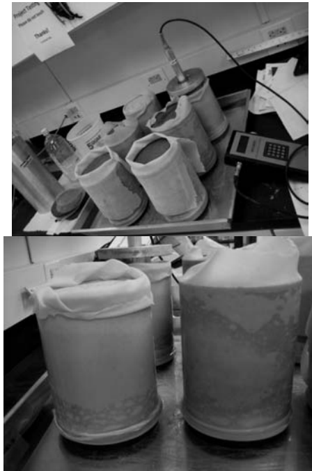
FIG.1. Illustration of the tube suction test using percolimeter
