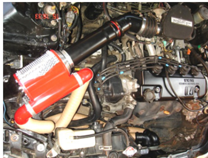
Figure 27. DATD, bi-route mounted on Honda Civic, 1.6
