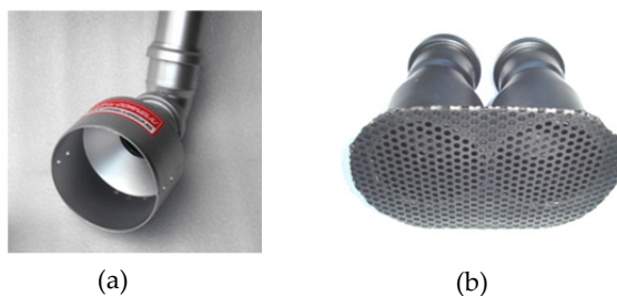
Figure 21. External collector diffusers - physical models
