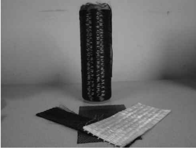
FIGURE 3.3 Carbon fiber yarn and carbon and glass fiber sheets used in strengthening.
