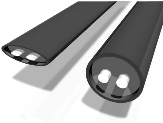
Figure 15 Mineral-insulated cable. On impact, all parts including the conductors are flattened, and a proportionate thickness of insulation remains between conductors, and conductors and sheath, without impairing the performance of the cable at normal working voltages
