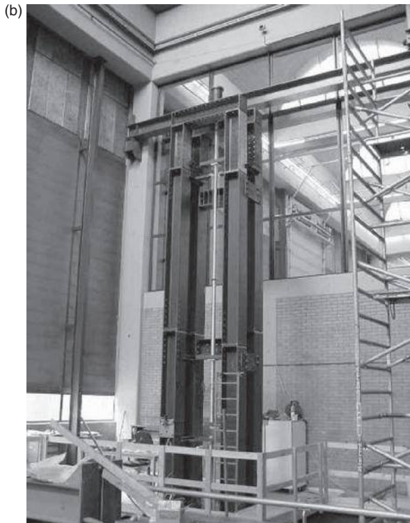
6.2 The SHB at Delft (a) measurement scheme; (b) set-up; (c) instrumented notched specimen.
