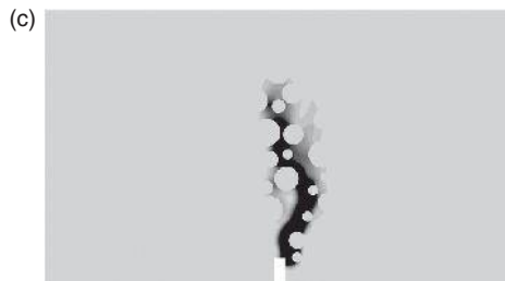
3.17 Effect of different bond thickness t_b in FE calculations: load-deflection curve and distribution of non-local strain measure close to notch: (a) t_b = 0.05 mm, (b) t_b = 0.25 mm, (c) t_b = 0.75 mm (small-size beam 80 \times 320 mm 2 , l_c = 1.5 mm, \rho = 45\% , gravel concrete with d_{50} = 2 mm and d_{\max} = 8 mm).
