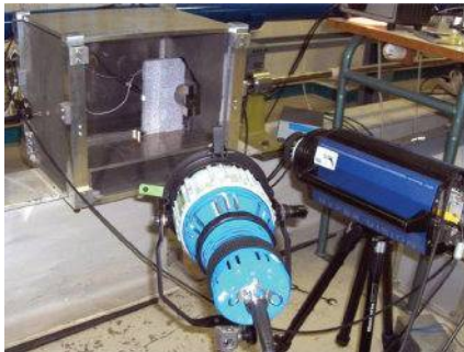
Plate X (Chapter 5) EOI experiments performed on concrete specimens in LEM3 lab. (Lorraine University) (Erzar, 2010) (a) Experimental set-up: gas gun, impact chamber, target and its confining system, UHS camera and lightening. (b) Far field measurement by DIC method: transverse displacement in pixel.
