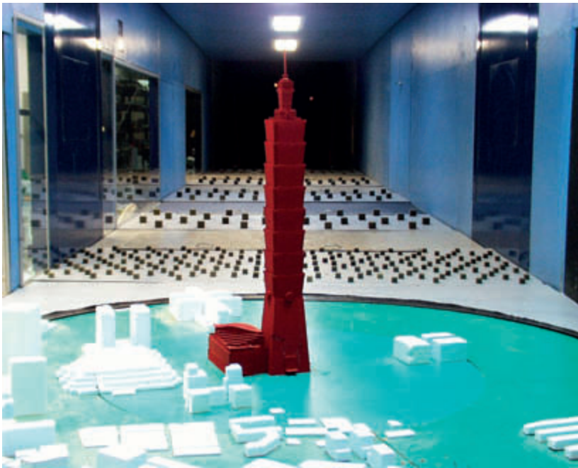
FIGURE 5.4 Taipei 101, wind tunnel test model (1:500 scale) (credit for photo: RWDI)
