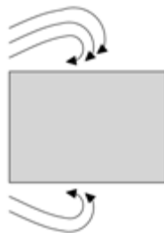
FIGURE 5.3 Vortices on along-wind sides of the building
