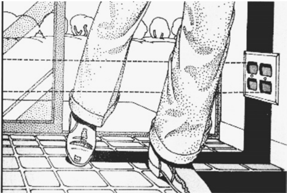
Figure 7.18 Transceivers and reflectors are located approximately 18 inches above the floor so that an intruder will break the beam.
