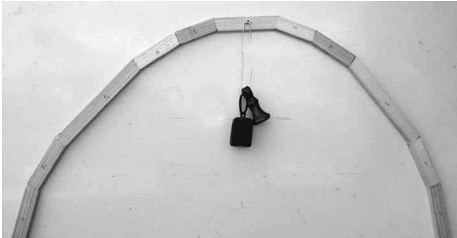
Figure 11.3: Photograph showing an inverted arch in compression.
