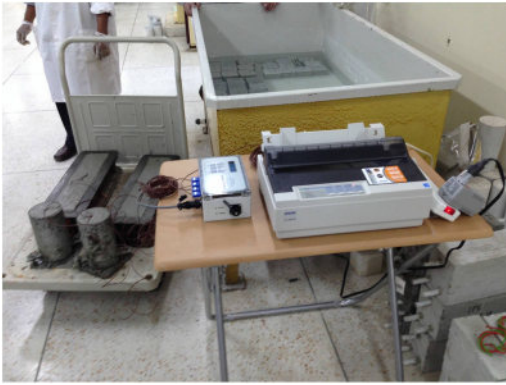
Plate 2. Connecting specimens to maturity meter.
