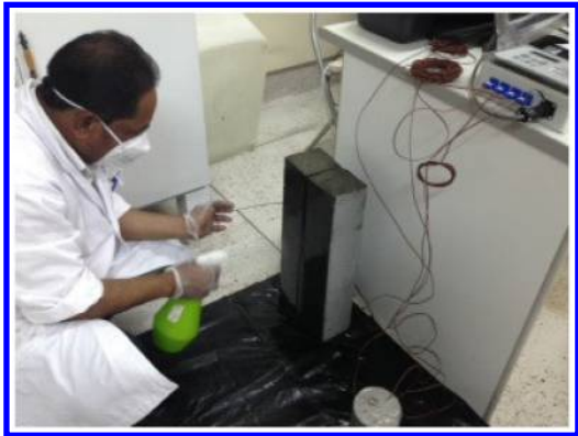
Plate 1. Application of spray coating curing.
