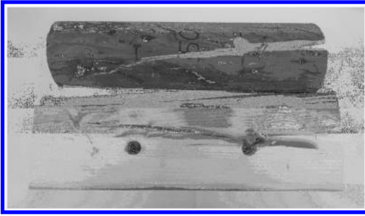
Figure 9. Disruption of round timber specimen in tension.
