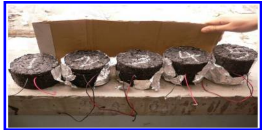
Figure 3. Marshall specimens with harvester in different burying depth.
