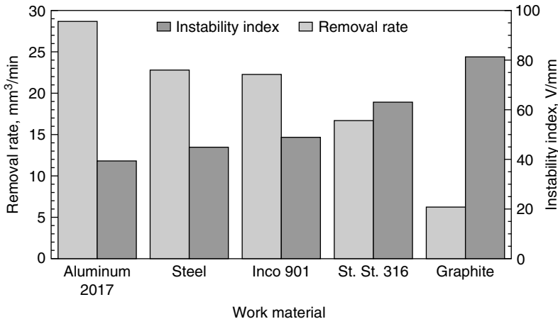
Figure 7.10 Machinability and stability in EEDM (El-Hofy, 1995).
