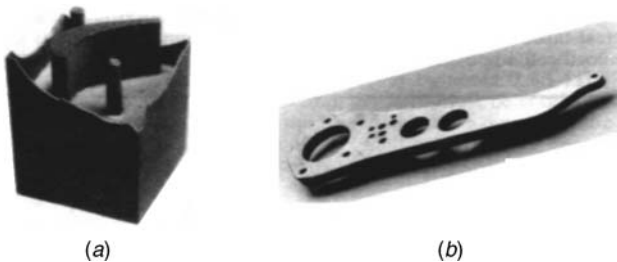
Figure 2.14 (a) Silicon nitride turbine blades (sinking), and (b) CFC acceleration lever and holes (contour USM) (Benkirane et al., 1995).
