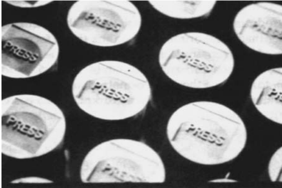
Figure 2.15 Graphite EDM electrodes machined by USM (Gilmore, 1995).
