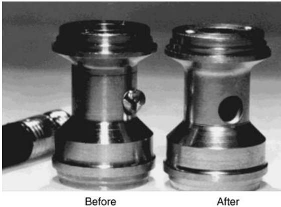
Figure 4.33 EC deburring applications (www.extrudhone.com/cation).
