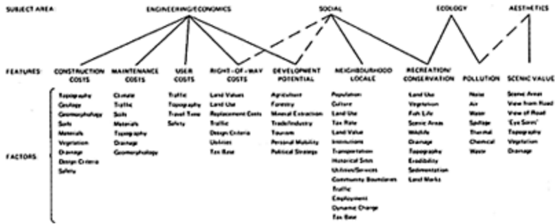
Figure 8.5 Factors affecting road alignment section (TRRL Supplementary Report 279, ref. 5).
