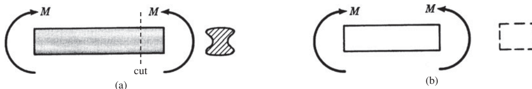
Fig. 7-2 A beam in pure bending.
