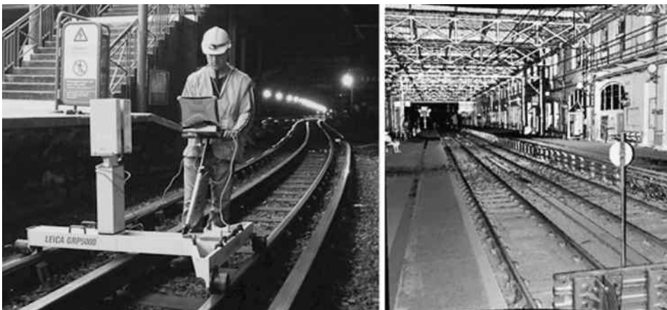
Fig. 14.43 Laser scanner on railway trolley and point cloud – courtesy of ABA Surveying
