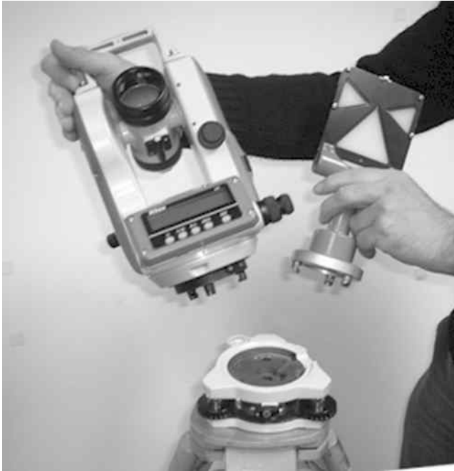
Fig. 6.16 Interchangeable total station and target with tribrach
