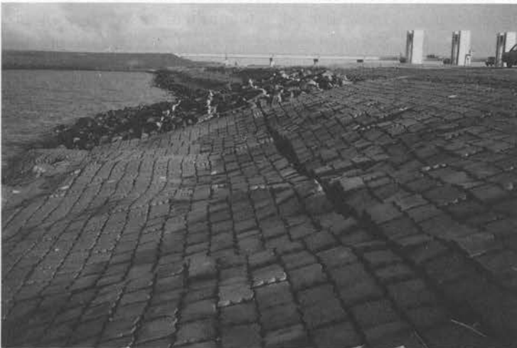
Figure 5.16 Damaged block mattresses at the test site near Lelystad at the IJsselmeer dike. Notice the fissure between the upper and the middle mattress, where the middle mattress has moved downward.
