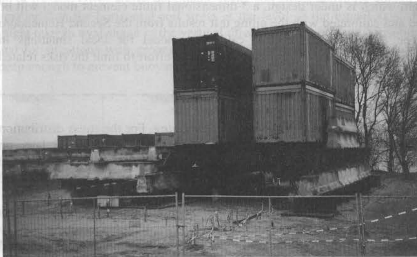
Figure 7.5 Test site for interaction Piled-foundation and tunnel boring at the site of the second Heinenoord tunnel
