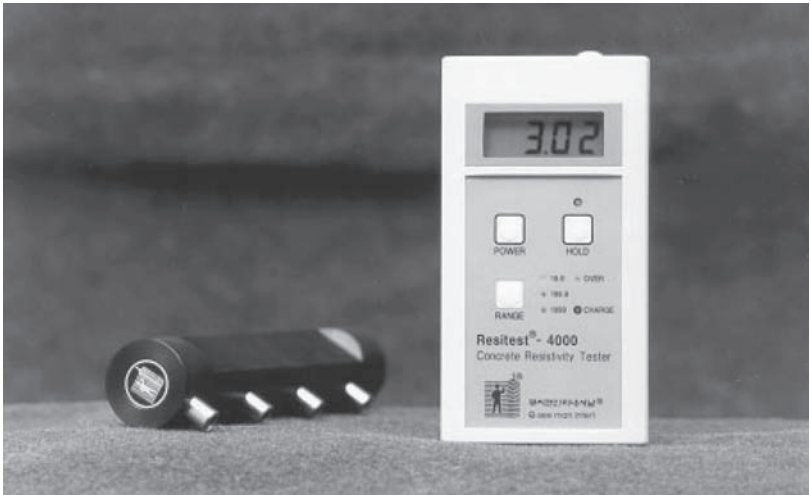
FIGURE 4.28 Electrical resistivity measurement equipment.
