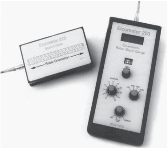
FIGURE 4.23 Concrete cover thickness measurement machine.
