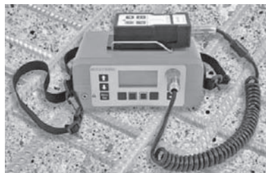
FIGURE 5.3 Electromagnetic cover meter.
