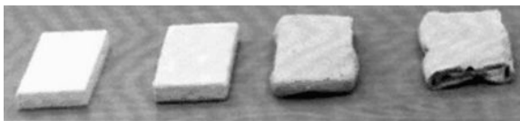
FIGURE 8.5 The EFPS samples: (a) sample without coating, (b) sample with coating, (c) and (d) samples after fire testing.
