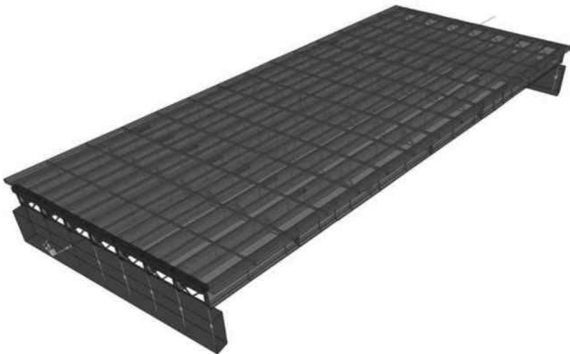
Figure 7.37 Global model of I-270 Middlebrook Bridge.
