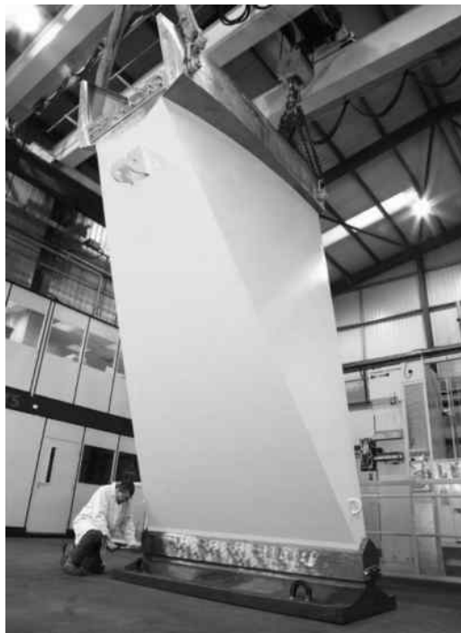
Figure 12.8 Flexible splay saddle as a rigid body (Hardanger Bridge, Norway).
